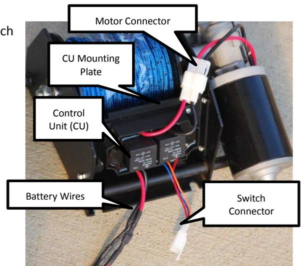
2. Install the Wireless Control Unit (CU) using the holes or slots that match the bolt pattern. (No drilling required.) Install Wireless CU with existing screws from the standard CU that was removed.
