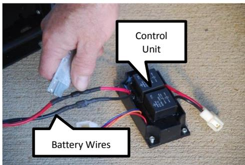
To disconnect the battery wires, first remove shrink tube. Cut with a utility knife. **DO NOT** cut fingers! Be careful.
